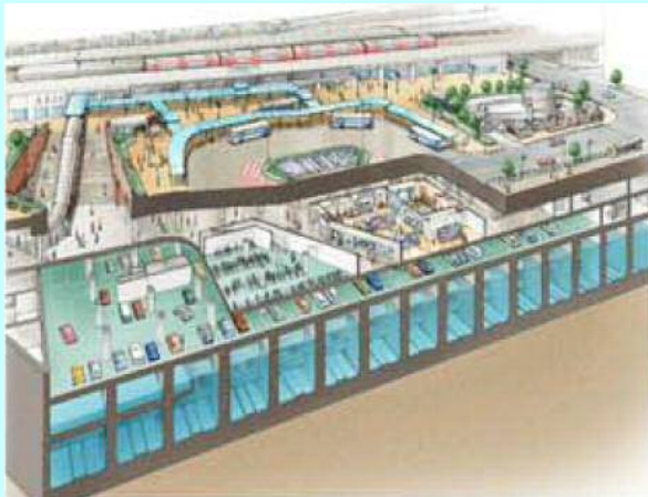
Ozone rain water Reservoir for pollution control
