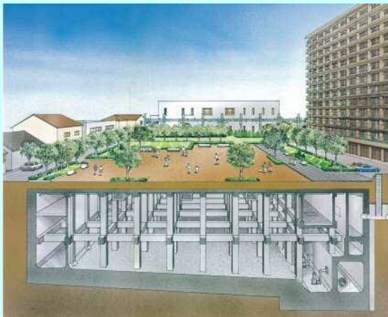
Takatuji Rain-water reservoir
