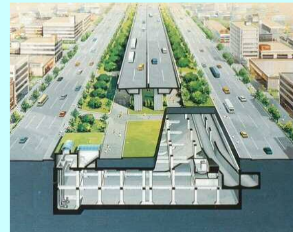
Improvement facilities of combined sewer system in Wakamiya avenue Rain-water reservoir
